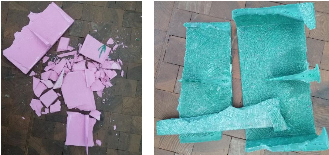
Figure 46 Break Fracture taken by Marina Seeger (left PP irradiated, right HDPE irradiated)
