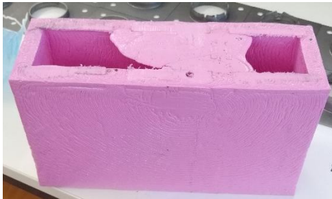
Figure 44 prepared Brick for Pressure Test (Marina Seeger)
