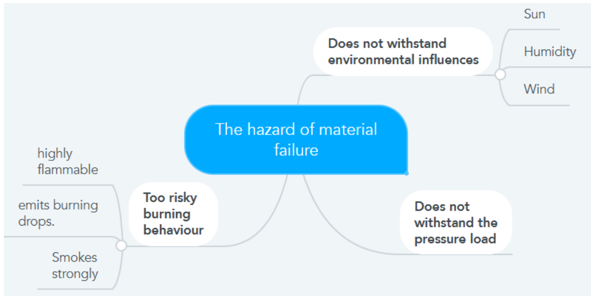
Figure 30 Overview of the hazard of material failure
