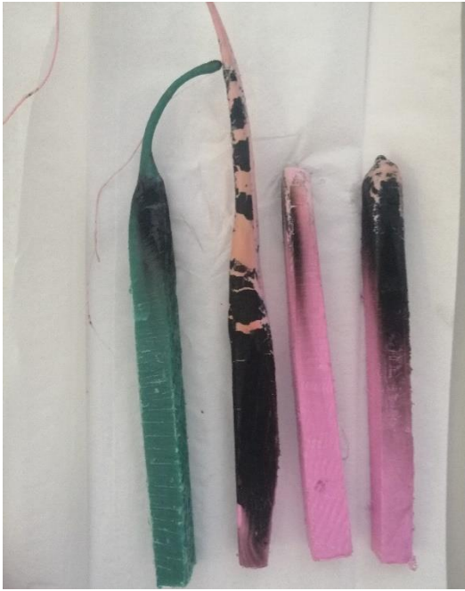
Figure 50 Test specimen after Test (from left to right HDPE_1; PP_3; PP_1; PP_2)
